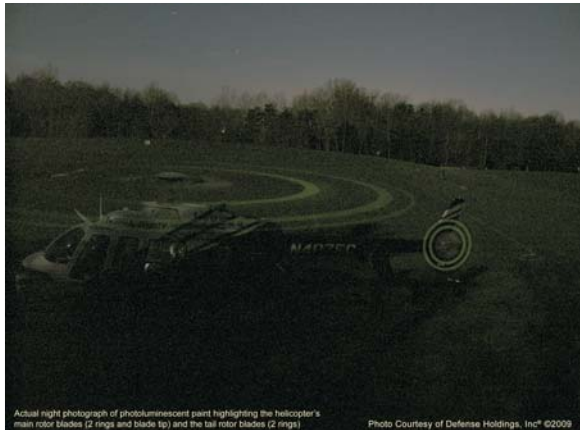
Actual night photograph of photoluminescent paint highlighting the helicopter's main rotor blades (2 rings and blade tip) and the tail rotor blades (2 rings). Photo Courtesy of Defense Holdings, Inc® ©2009
